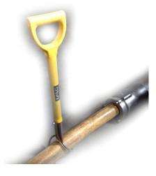
For example, a shovel operator is able to use bucket to lift and relocate cable that is attached to the Viking, and thus preventing cable damage typically resulting from cable being dragged behind equipment when equipment is relocating.
