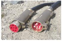
1.1kV couplers are typically used in hard-rock mining or tunnelling operations. They are used to distribute power to electrical site equipment such as shovels, drillers, pumps, controllers, motors & such. Couplers area available in: 170A or 250A rating; Aluminum or Bronze housing; powdercoated or bare metal; 1 or 2 Control/Pilot Pins; Cable-mount or Equipmentmount style
